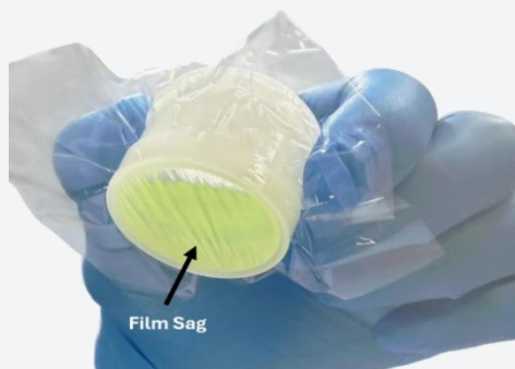
Figure 3 —Chemical Resistance of Diesel Fuel using 4.0 \mu\text{m} Polypropylene Film
